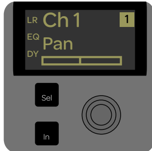
Channel encoder, Sel and In switches, and display (Input Channel shown)
