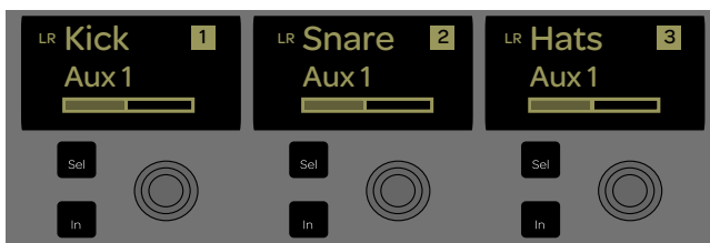
Channel encoder Sel switch (top) and In switch (bottom)
