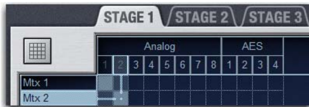
Assigning a Matrix mixer output to a Stage IO box hardware output
