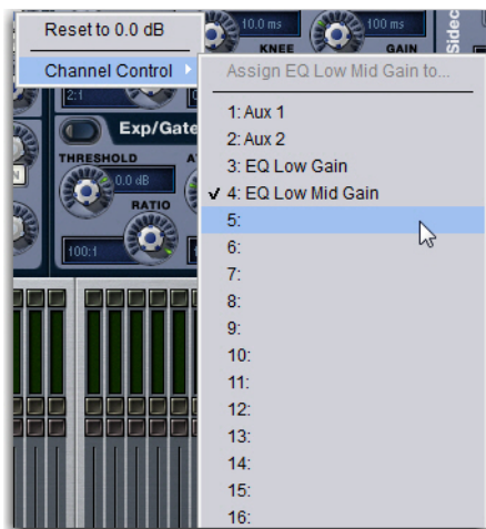
Assigning a parameter to Channel Control on-screen
