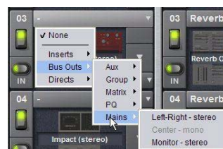
Assigning monitor output to a bus-fed plug-in
