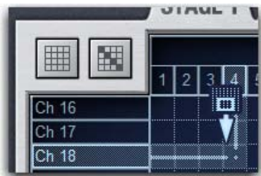
Scrolling the Patching Grid by right-clicking and dragging
