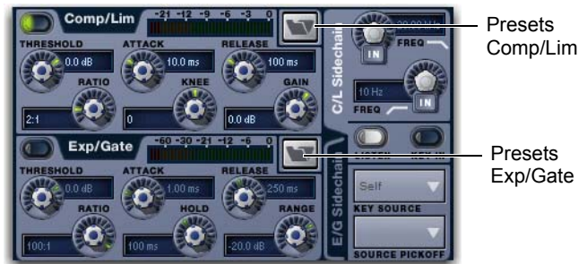
Built-in dynamics Presets buttons
