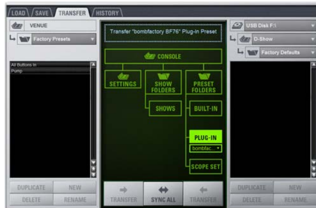
Preparing to transfer items to a USB storage device
