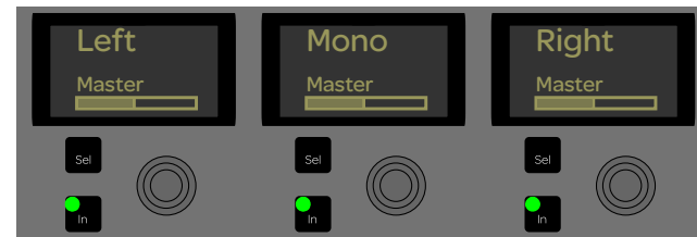
Main busses assigned to the Global Control encoders
