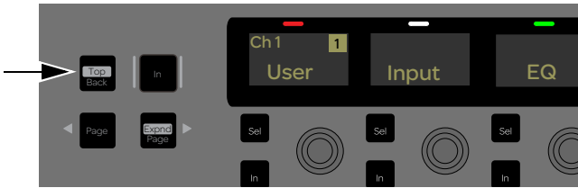
Back/Top Channel Control Navigation switch
