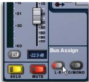
Assigning a Group output to the Mains from the Output page
