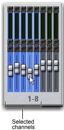
Dragging multiple faders on-screen
