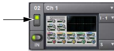
Rack slot power switch
