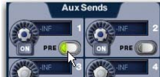
Activating Pre pickoff for an Aux Send (Inputs page shown)
