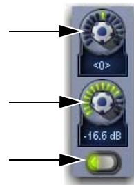
On-screen Matrix input pan control knob (top), level control knob (middle) and On button (bottom)
