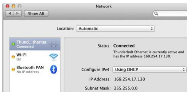
Mac Network Settings screen showing an active network connection to the S3L-X system
