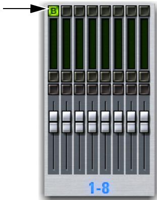
On-screen Channel Safe switch indicating the channel is Bank Safed
