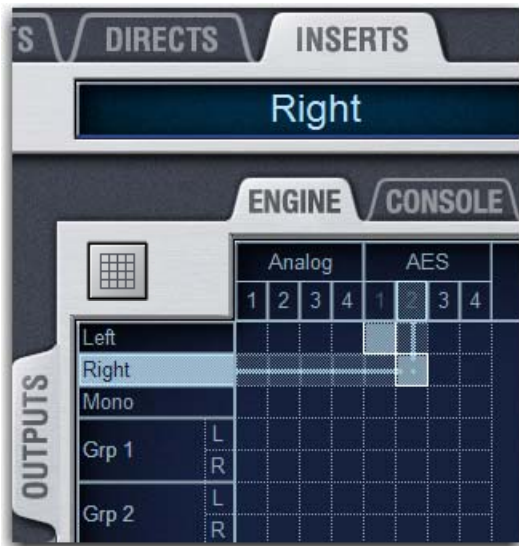
Assigning a hardware insert on the Inserts tab of the Patchbay I
