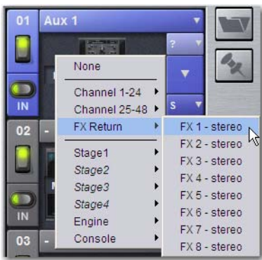
Assigning plug-in output to an FX Return
