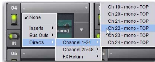
Assigning a channel Direct Out as a plug-in input source in the Plug-Ins page
