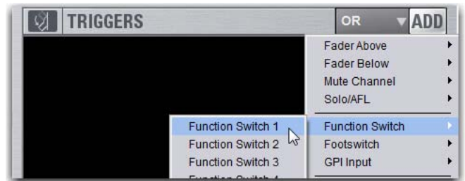
Selecting a Function Switch from the Triggers list
