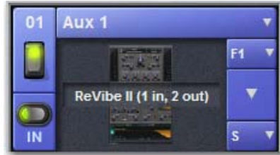
A bus-fed plug-in shown in the rack
