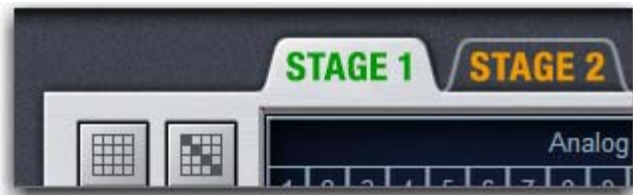
Stage tabs showing Master (left) and Slave (right) statuses on the Patchbay page
