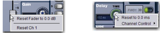
Right-clicking channel strip controls on-screen
